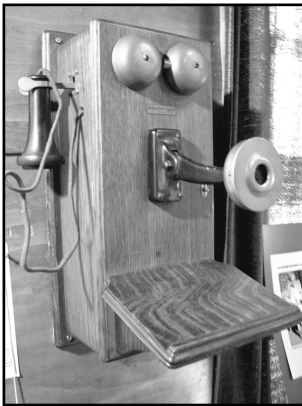
The Lymbery family's battery-powered magneto phone. All calls went through a central operator in Nelson until 1963, when BC Tel finally introduced dial phones to our area. Photo: Frances Roback, 2010
