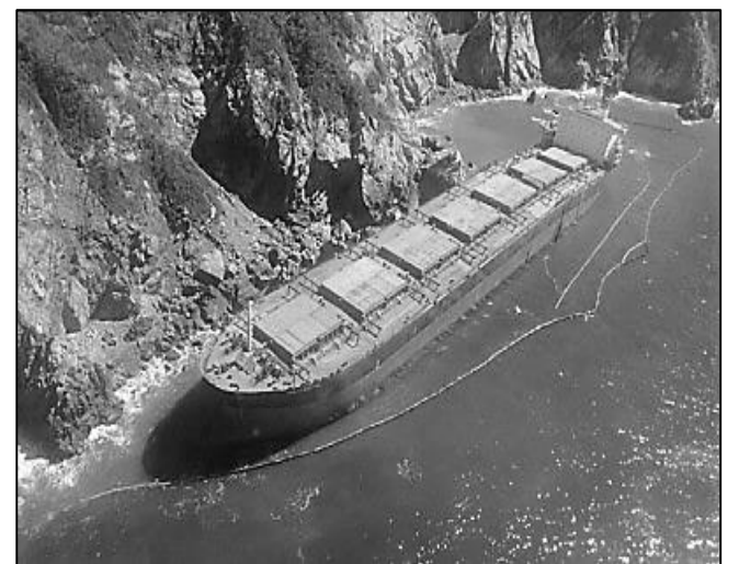
This photo doesn't show the enormous size of MV Los Llanitos - the stern of the ship is at the far right with its bridge and accommodation towering above the seven tremendous holds where bulk cargo can be stored.
