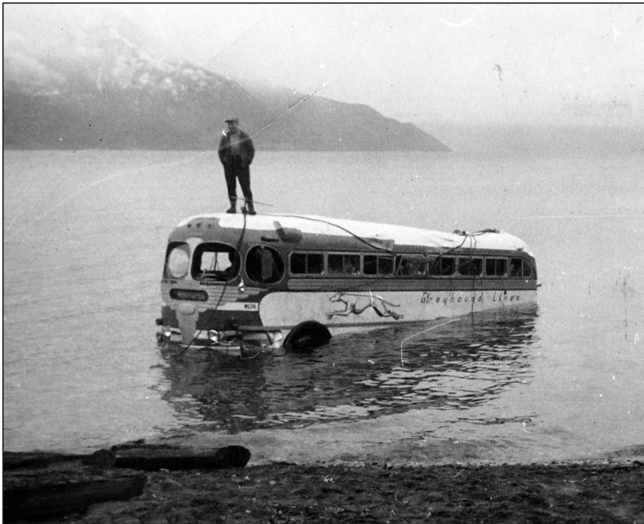
Hauling the Greyhound bus from Kootenay Lake at La France Creek (Mountain Shores), Dec. 1952. After skidding off the road and down a 100' embankment, the bus landed on its side in the lake. It was set back on its wheels, filled with inner tubes for buoyancy, hitched to long cables, and pulled through the water to the beach with a Caterpillar tractor operated by Bert Learmonth. Nelson Greyhound mechanic Roy McKay guided the steering from the roof of the bus. Photo courtesy of Mary Carne (Greyhound photo album)
