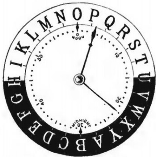
Sandford Fleming's proposed 24-hour world clock, using letters for the earth's meridians instead of numbers.
