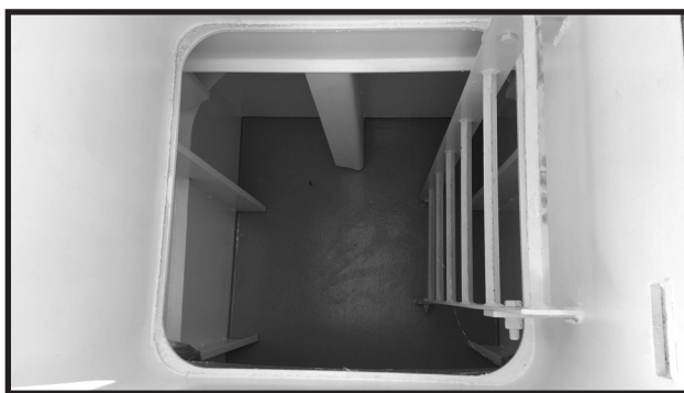
One of the four hatches on the car deck is open to show the ladder used by the ferry crew to go down to or up from the engine deck. Certainly not an "escape hatch slide" for passengers. Photo courtesy of Dave Lymbery
