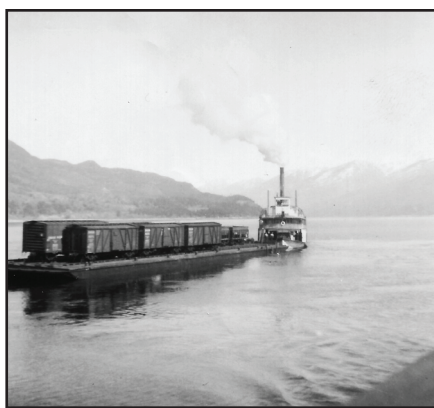
A railway barge loaded with baggage cars is pushed across Kootenay Lake by the SS Moyie , 1920's. Photo: GCHS (Don Karpowich)
